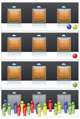
Destination dispatching results in a low mix of destinations per car, requiring fewer stops and taking far less time.
