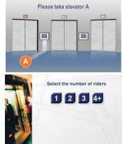
MCE touch-screen technology provides highly visible, on-screen operating panels and allows unique customer options to be easily implemented. After a destination selection is entered, the screen displays a map for easy elevator location. Entry screens can switch to conventional up/down button entry for conventional operation on a timed or user input basis.
