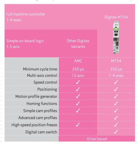
The powerful MCi second processor onboard of Digitax M754 extends the drive's system and machine control capabilities to run application programs up to four times faster than a standard PLC.
