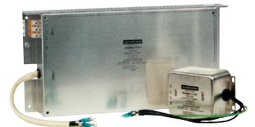
Output filters change the drive's output to the motor thus creating less stress on the motor windings. This filter can be a simple reactor, a dV/dt filter or a sine filter.
