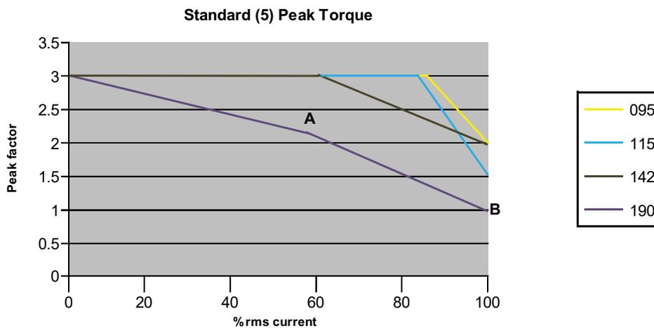
Peak torque is defined for a maximum period of 250ms, rms % rms = % rms duty cycle Current for motor in application
