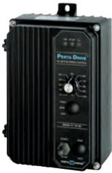
The KBPW-240D DC Drive is a Pulse-Width Modulated (PWM) control housed in a NEMA 4X / IP 65 washdown/watertight enclosure for indoor or outdoor use. It is designed to operate Permanent Magnet and Shunt Wound motors from 1/100 to 2 horsepower.
