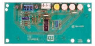
The PID Module is a factory installed option that enhances the dynamic and steady state response of the KBRG. The unit can be adjusted for precise settings of frequency band width and gain. It eliminates "hunting" and error in dancer arm applications, such as feeders and winders. Four independent trimpots provide a wide range of adjustment for frequency bandwidth and gain.
