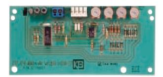
The 4-Quadrant Accel/Decel Module provides independent adjustment of forward acceleration, forward deceleration, reverse acceleration and reverse deceleration. An individual trimpot is provided for each adjustment mode. The Module also contains a dual time range which is jumper selectable over a time period of .3 seconds and .3 to 30 seconds.
