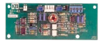
The SI-4X provides complete electrical isolation between input voltage signals which are derived from programmable controllers, transducers and digital/analog converters and the KBRG. The Module contains two input ranges (±25, ±250 VDC) which are jumper selectable. The input/output ratio can be scaled via the included "ZERO" and "MAX" trimpots. The SI-4X installs easily onto the KBRG chassis.
