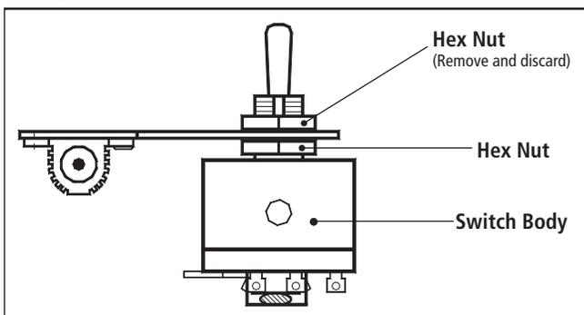
Figure 2 – FWD-BRK-REV Switch After Installation
