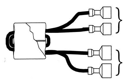
Female (0.25") Quick Connect Terminals To DC Drive Output Terminals.
