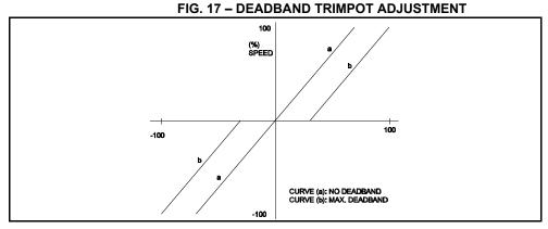
The DB trimpot also determines the amount of delay that will occur before regeneration starts. Regeneration occurs when the applied load torque is in the same direction as the motor rotation.
