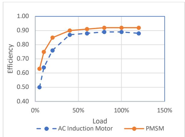
Figure 1: Typical AC Induction Motor vs PMSM Efficiency
