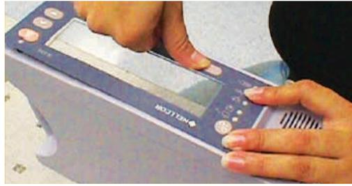
**Figure 6b:** NEVER burnish switch during assembly; it can inadvertently damage dome legs and/or SMT LEDs conductive pads.
