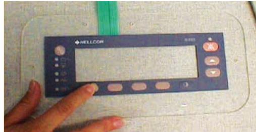
**Figure 2b:** Detail view: tactile membrane switch is laying flat in proper test fixture during test key actuation.
