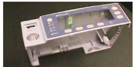
**Figure 12:** Finished part laminated to typical customer casing. Membrane switches may ONLY be laminated to substrate ONE time. VIS can not warranty parts that have been removed and/or repositioned for final assembly.
