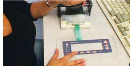
**Figure 2a:** Parts are tested prior to assembly. Note tactile membrane switch is laying flat in proper test fixture.
