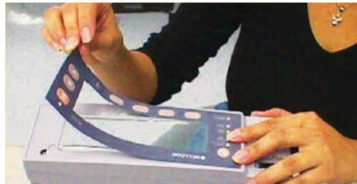
**Figure 5b:** NEVER roll the membrane switch onto casing or wellmount on bezel.
