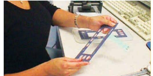
**Figure 3a:** NEVER actuate keys in unsupported position. Tactile membrane switches should ALWAYS be tested in flat (and supported for component clearance) position.
