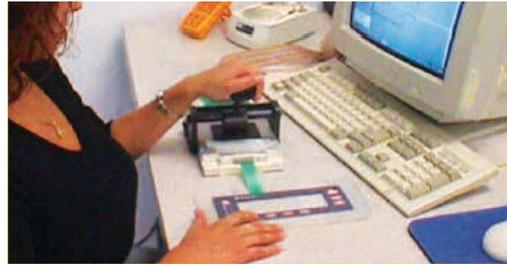
**Figure 1:** Recommended test setup. Switch tester measures: circuit continuity, closed-circuit resistance, LED polarity and function.
