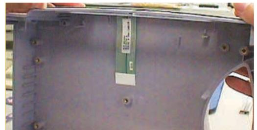
**Figure 8:** Detail side view: showing 0.040" polycarbonate template matching curve of well-mount in plastic casing.
