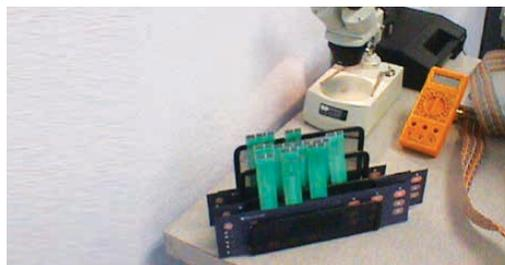
**Figure 11:** Detail view: showing membrane switches stacked vertically for testing prior to assembly. Never place objects on switches in unsupported manner.
