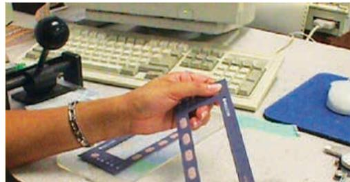
**Figure 3b:** NEVER actuate keys in unsupported position.
