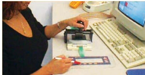
**Figure 4b:** NEVER actuate keys with any hard object. During test or in field operation.
