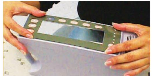
**Figure 7c:** After threading tail through slot, PSA is exposed and placed (in flat plane, not rolled) onto well-mount on plastic case.
