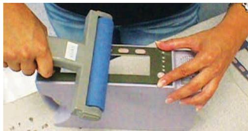
**Figure 9:** Using template, laminate membrane switch with smooth even pressure of hand-roller (typ. 40-45 Durometer, shore A)
