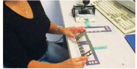
**Figure 7a:** ALWAYS use laminating template to apply switch assembly.
