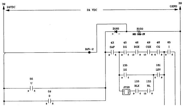
6. On sheet 7, line 71 of the wiring diagrams, remove the existing 'BK' contact. Referring to the diagram below, wire 'PRV' #9/5 and 'PRV' #6/10 in the 'M' relay circuit.
