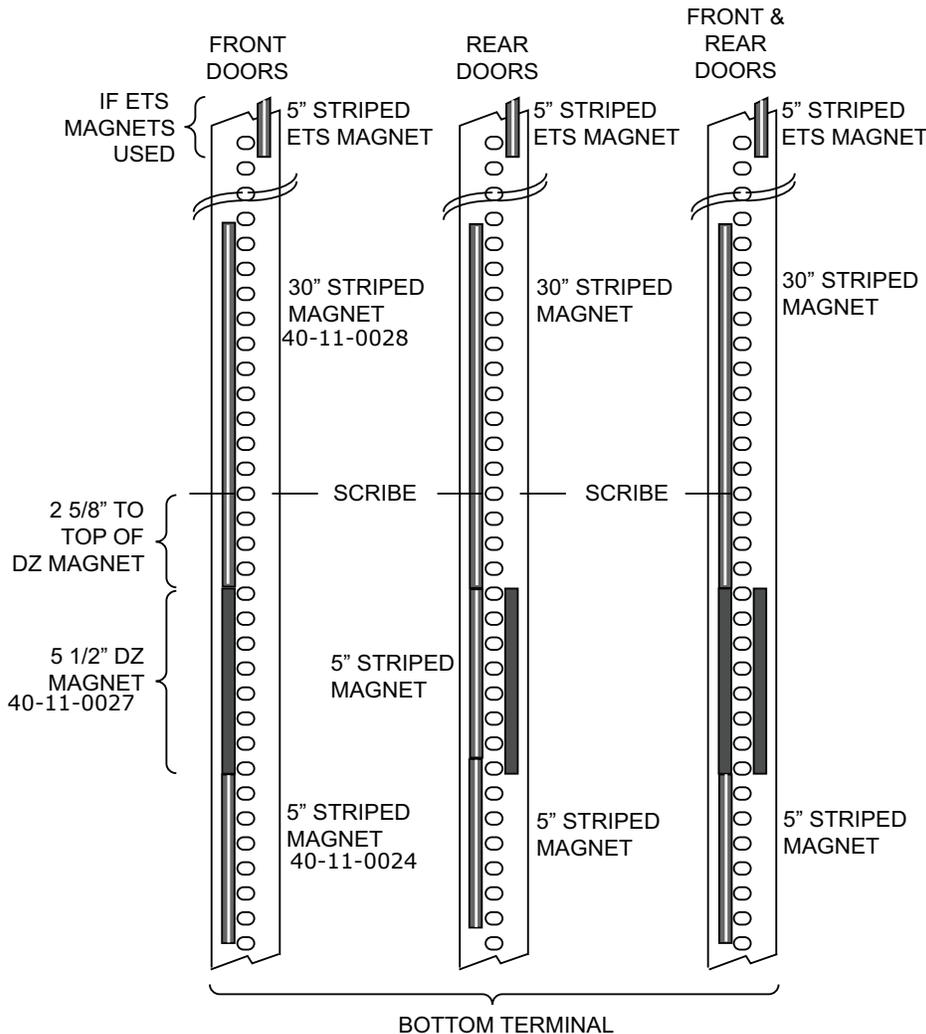
1. Place a 30-inch, striped magnet on the tape to the left of the holes, just above the bottom door zone magnet as shown above. The bottom of the 30-inch magnet must be even with the top of the door zone magnet.
