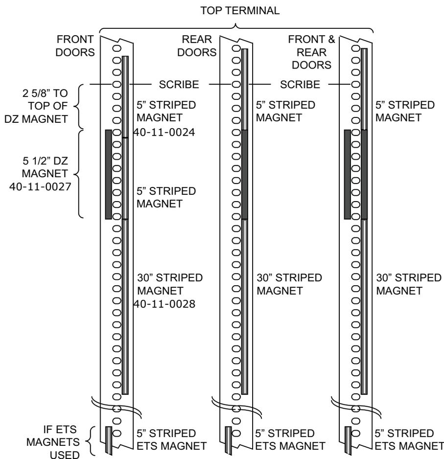
1. Place a 30-inch, striped magnet on the tape to the right of the holes, just below the top door zone magnet as shown above. The top of the 30-inch magnet must be even with the bottom of the door zone magnet.
