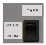
The BYPASS switch above is not visible unless the TAPS cover is removed
