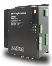
The DVR100T digital voltage regulator provides brush-type excitation control for alternators in locomotive traction applications. It utilizes a current mode pulse width modulated output that can be sourced from a battery or other DC supply. This regulator is essentially a "buck" type regulator that can deliver up to 96% of the source voltage to the load.
