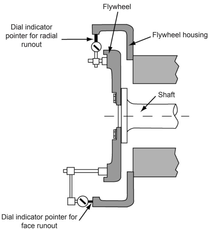
**Figure 2-1: Flywheel housing check**
