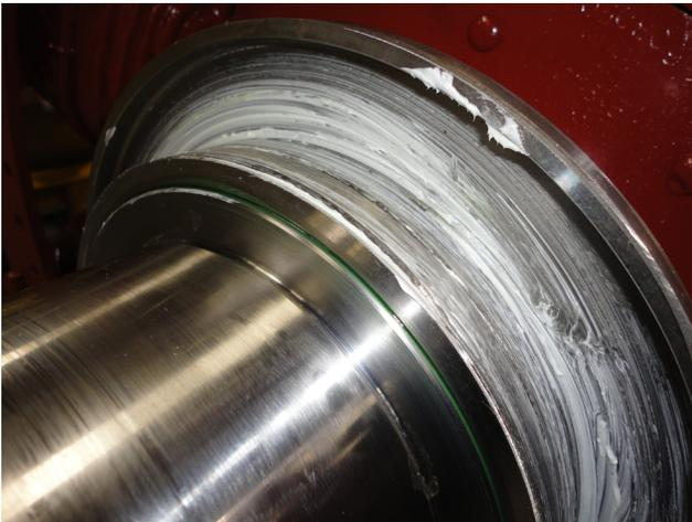
*Figure 5-4: Inboard slinger*
