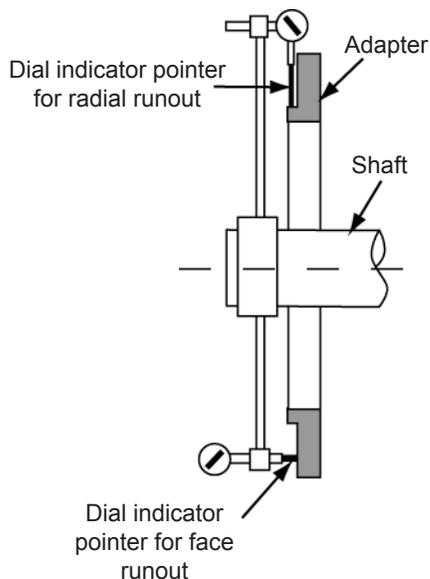
**Figure 2-3: Generator adapter check**
