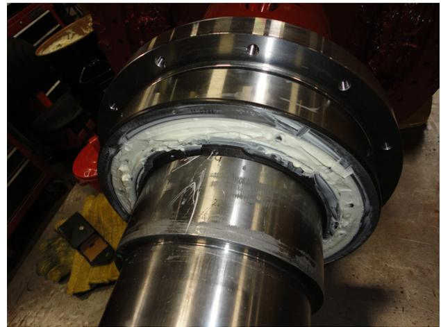
*Figure 5-6: Bearing Installed on Shaft*
