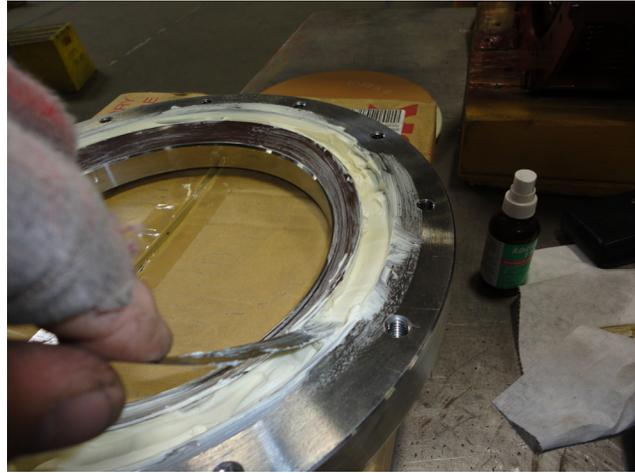
*Figure 5-5: Applying grease*
