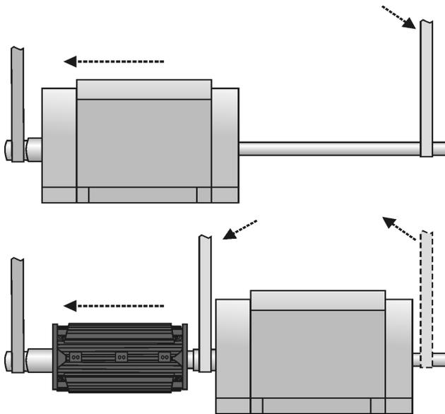
*Figure 5-7: Rotor Removal*
