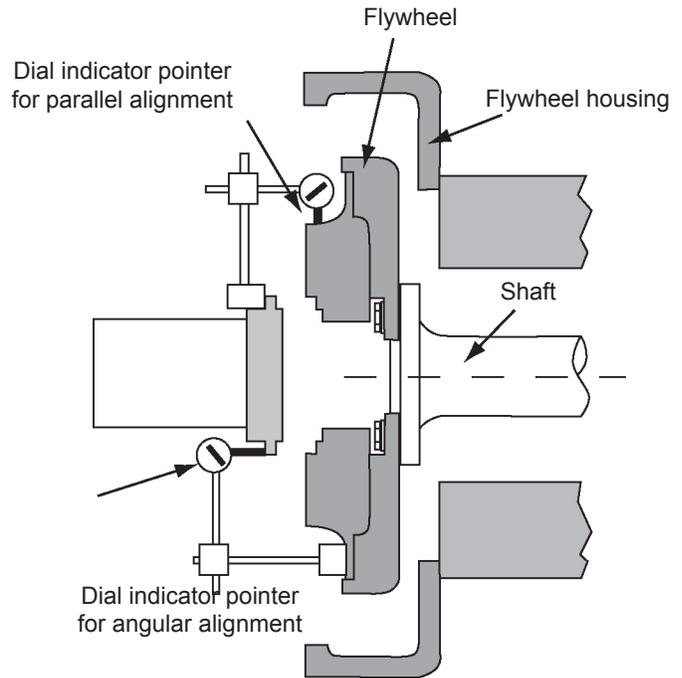
**Figure 2-4: Alignment check**
