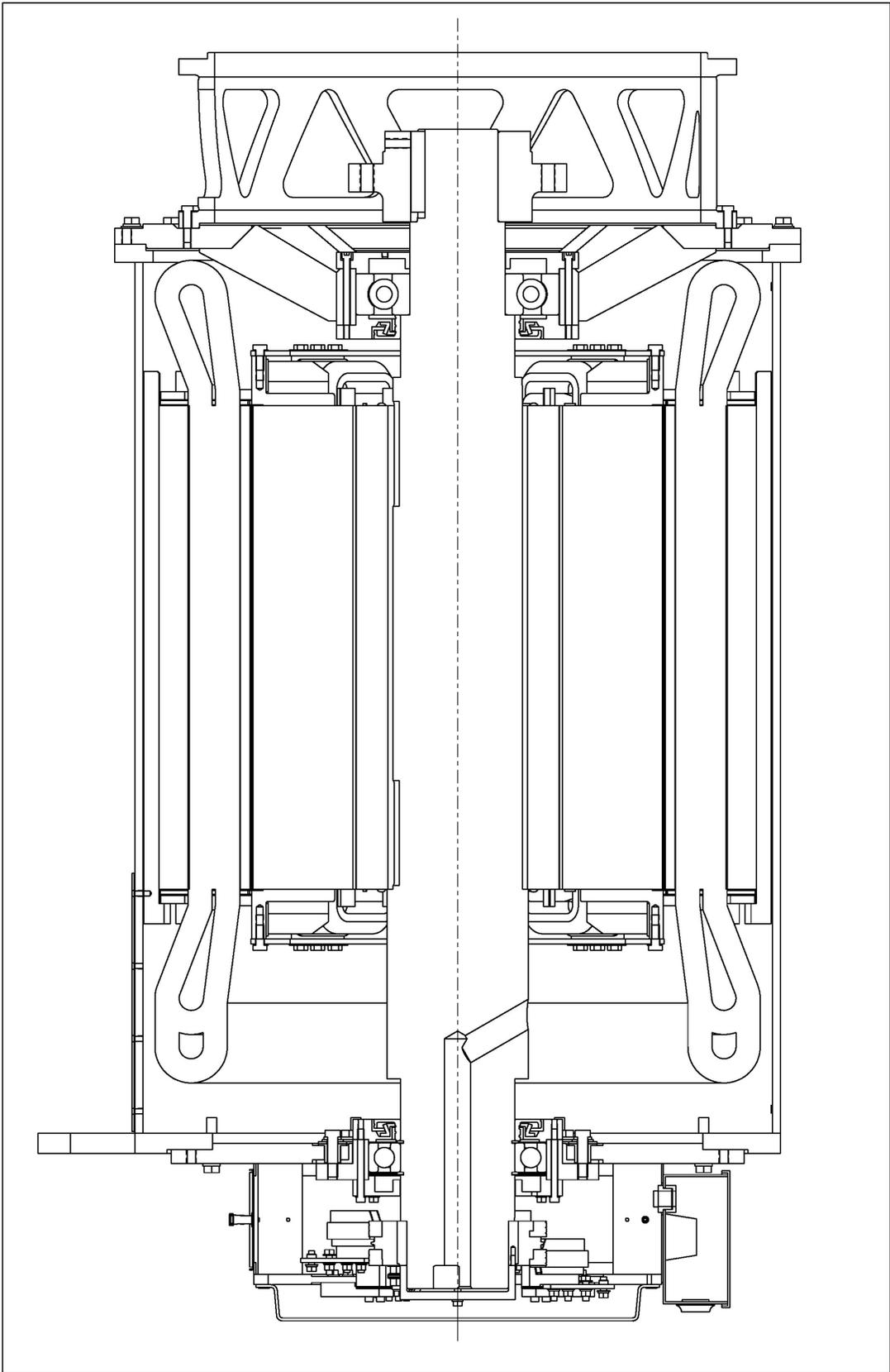
*Figure 5-1 Cut Away View Of Traction Alternator*
