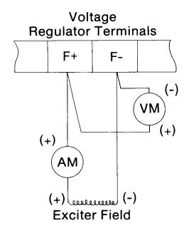
NOTE: Use dc voltmeter and dc ammeter with scale equal to or more than the oneminute field forcing capacity given in the voltage regulator instruction manual.
