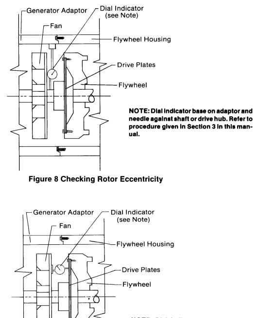
NOTE: Dial indicator base on fan and needle against drive plates. Refer to procedure given in Section 3 in this manual.
