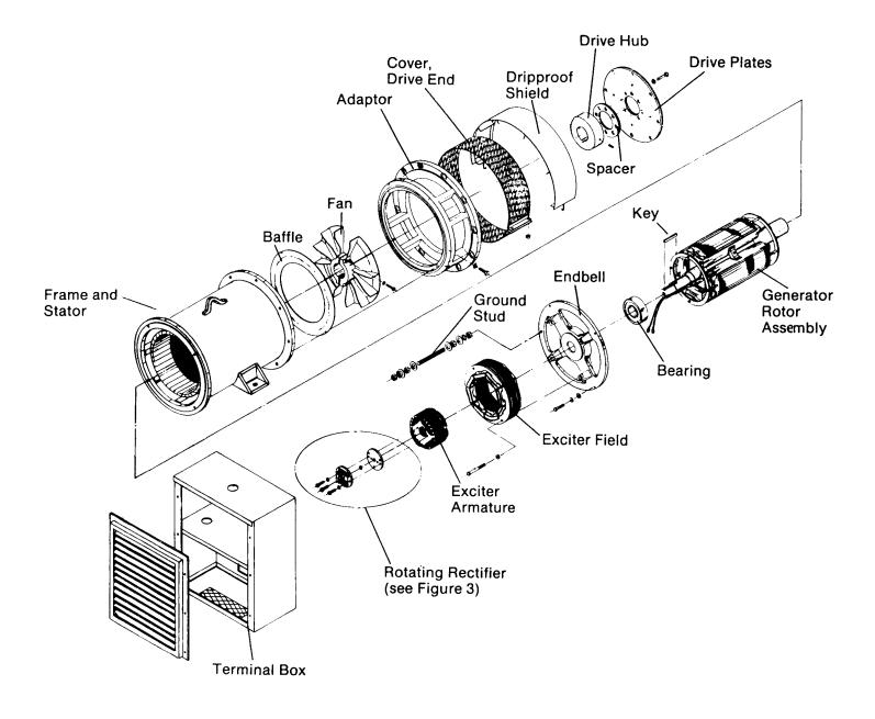
Figure 1 Single Bearing Kamag Generator With Outboard Exciter
