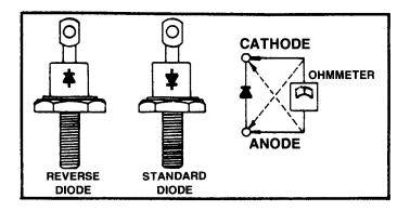
Figure 13 Testing Rotating Rectifiers with an Ohmmeter
