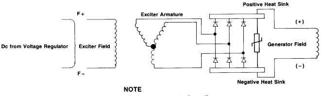
Three forward polarity diodes are mounted on the positive heat sink, and three reverse polarity diodes are mounted on the negative heat sink. A surge suppressor is mounted across the heat sinks.
