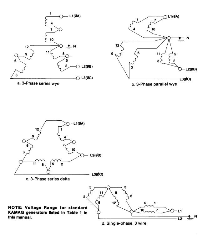
Figure 10 Twelve Wire Generator Stator Lead Wire Connection Diagram
