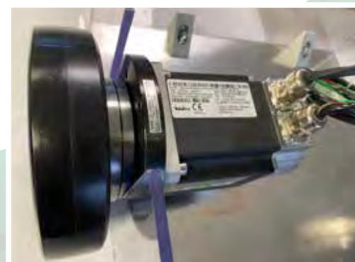
Mounted from inside the AGV, the bolts go through the motor mounting plate from the rear and attach to the inside of the AGV body. Take care in leaving enough clearance between the AGV motor wheel and the AGV body.
