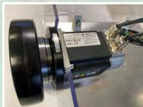
Mounted from outside the AGV, the bolts go through the motor mounting plate from the front and attach to the outside of the AGV body. This does not affect the clearance between the AGV motor wheel and the AGV body.
