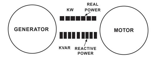
Illustration of an SCIM under partially loaded conditions without Power Factor Correction Capacitors (PFCC).
