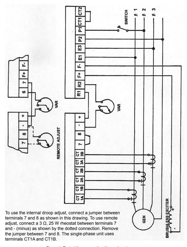
Figure 1: Typical line connection (three phase)
