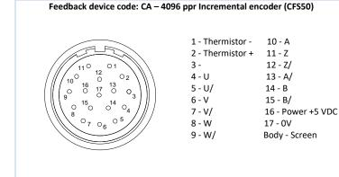
Connection type: B – Power and Signal 90° rotatable (Size 1)
