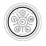
Connection type: B – Power and Signal 90° rotatable (Size 1)
