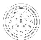
1 - Thermistor -10 - A 2 - Thermistor + 11 - Z 3 -12 - Z/ 4 - U 13 - A/ 14 - B 5 - U/ 6 - V 15 - B/ 7 - V/ 16 - Power +5 VDC 8 - W 17 - 0V 9 - W/ Body - Screen
