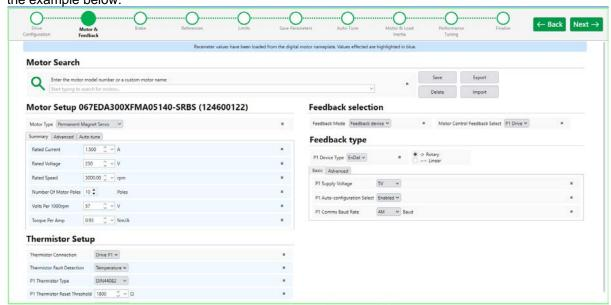
The light blue highlight shows that the electronic nameplate has been loaded. In addition, for EnDat 2.2, EnDat 3.0 and BiSS-C encoders the "Encoder type" fields are also configured automatically.
