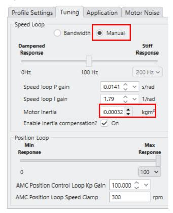
**HINT:** If the Inertia has been modified to tune the output of the Inertia Compensation feature, and Bandwidth mode tuning is later required, the inertia must be restored to its original value before selecting bandwidth mode, otherwise the speed loop gains may be calculated incorrectly.
