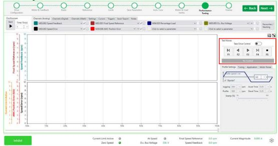
Commissioning tabs – configure the test move motion profile, speed and position loop tuning, application optimisation controls, and motor noise optimisation controls.
