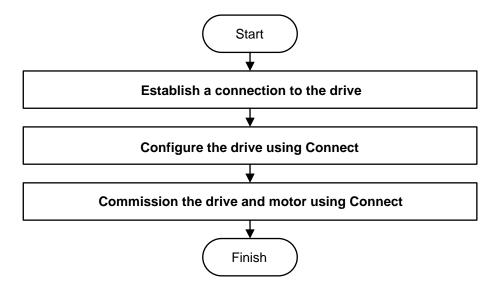
The end result is a Control Techniques drive that has been configured as per the users requirements and commissioned with a motor tune that is best suited to the application, i.e. biased towards low acoustic noise, or biased towards a dynamic response at the cost of higher acoustic noise levels.
