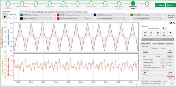
Care must be taken when increasing the gain as it is possible to increase the gain until the system stability limit is reached and the axis motor will make additional noise or worst case oscillate. Small steps are recommended when tuning.
