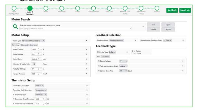
The user must configure the motor, feedback device and thermistor setup here.
