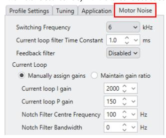
For most applications it is recommended to use a Current Loop Filter Time Constant of 1.0ms, unless the application is ultra-dynamic and needs a very fast response where a lower value is needed. A 1.0ms filter gives a 160Hz response bandwidth, where most systems will be well tuned at between 50Hz and 100Hz.
