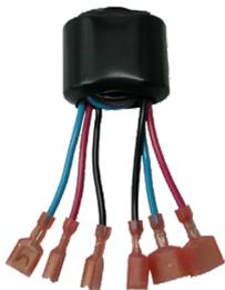
RFI Filters are used to suppress electronic interference caused by motor speed controls. They have been designed to limit the interference to within acceptable levels as determined by the CE Council Directive 89/336/EEC relating to the Class A Industrial Standard and Class B Residential Standard. The AC Line / DC Motor Choke is used to provide supplemental RFI filtering, if required. Maximum current rating is 14 Amps.
