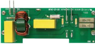
The RFAC Line Filters are used to suppress electrical interference within acceptable levels as determined by the CE Council Directive 89/336/EEC relating to the Class A Industrial Standard. The RFAC-24D (Item number 9507) is rated for 10 Amps at 230 Volts AC. The RFAC-27D (Item number 9512) is rated for 22 Amps at 230 Volts AC. Both filters can be used with or without the On/Off AC Line Switch Kit.
