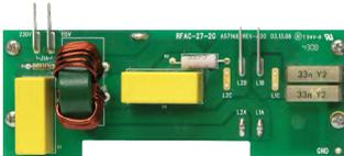
The RFAC Line Filters are used to suppress electrical interference within acceptable levels as determined by the CE Council Directive 89/336/EEC relating to the Class A Industrial Standard. The RFAC-3PS (Item number 9479) is rated 10 Amps at 460 VAC and requires the On/Off AC Line Switch Kit. The RFAC-3PNS (Item number 9515) is rated 10 Amps at 460 VAC does not require the On/Off AC Line Switch Kit.
