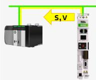
**Safe Value Transfer** safe position and speed value transfer over safety fieldbus for further processing by safety controller
