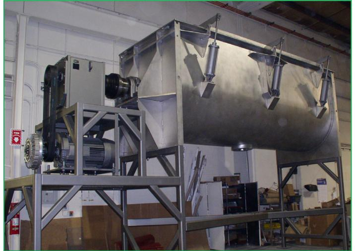
The recipe should include mixer speed throughout the mixing process. Optimal speed will likely change according to the consistency of the mixture and will directly affect product quality and production throughput.
