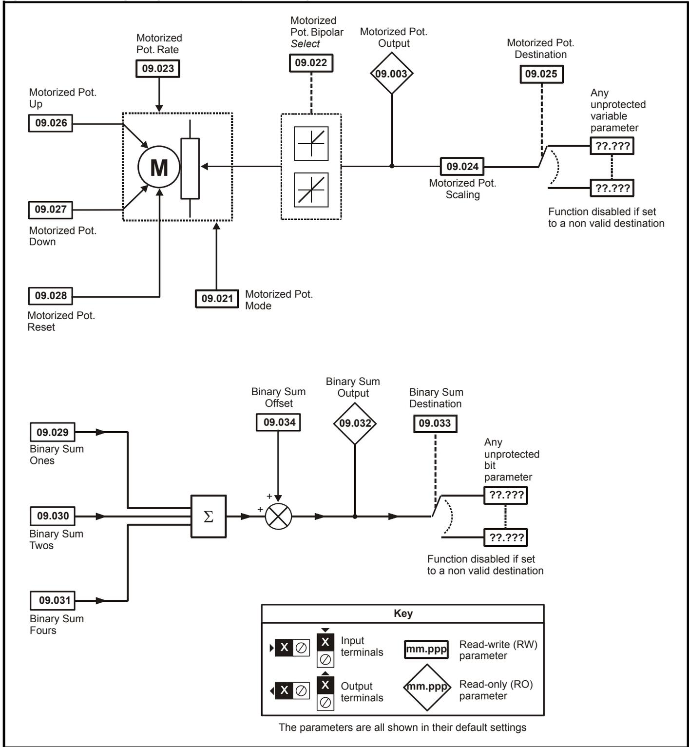
Figure 11-18 Menu 9 logic diagram: Timers
