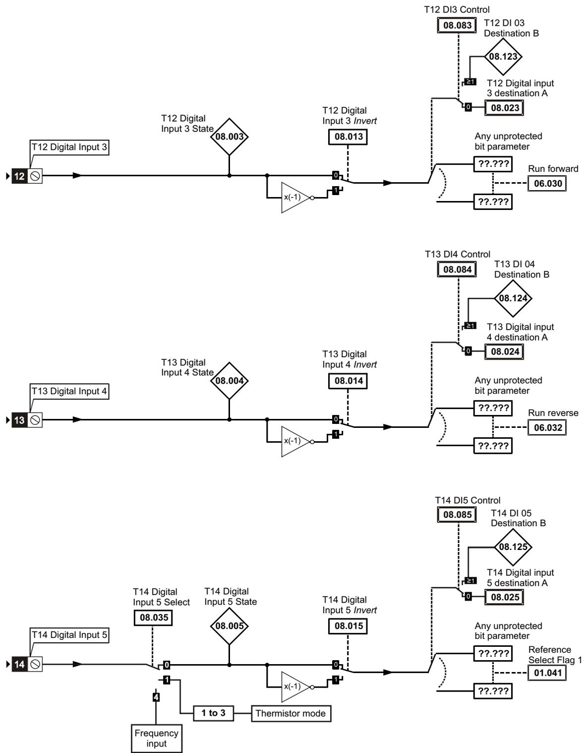
Figure 11-14 Menu 8 logic (relay)
