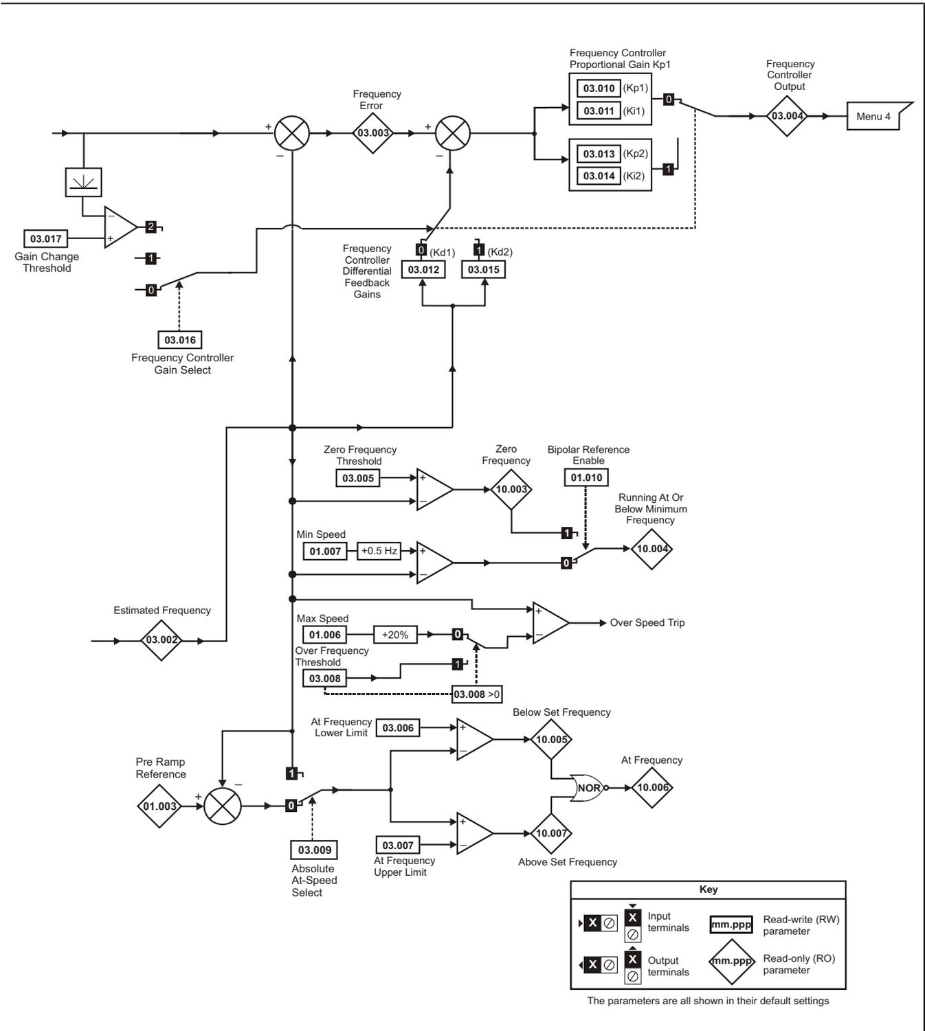
Figure 11-5 Menu 3 logic diagram
