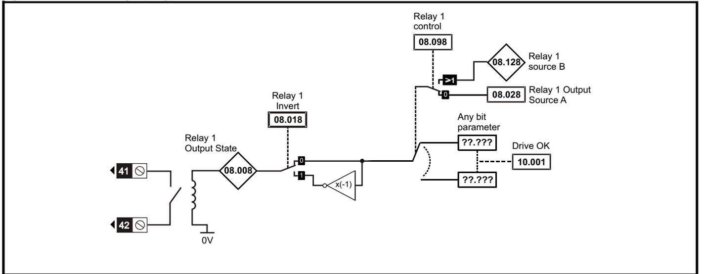
Figure 11-15 Menu 8 logic (Remote Keypad RTC)
