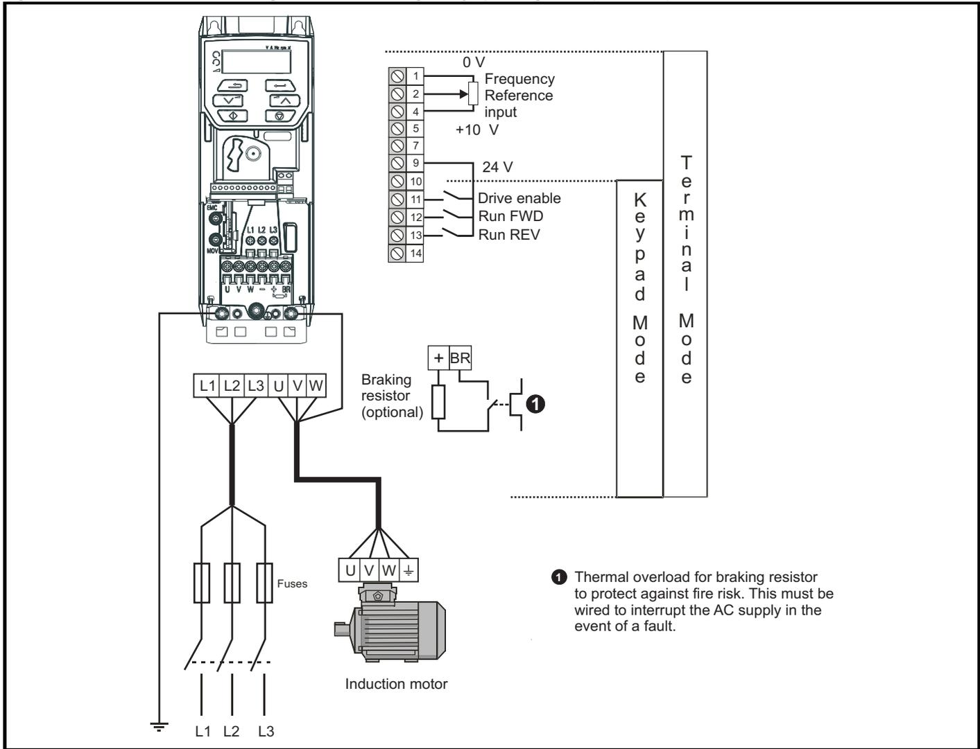
**Figure 7-2 Minimum connections to get the motor running in any operating mode (size 5)**
