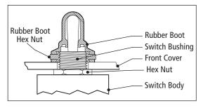
Figure 2 – Jumper Assembly
