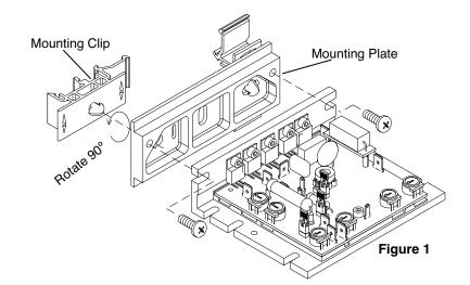
**Caution**: Do not overtighten mounting plate screws.
