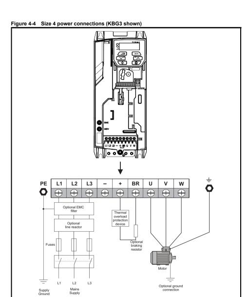
See Figure 4-5 Size 1 to 4 ground connections (KBG3 size 2 shown) on page 42 for further information on ground connections.
