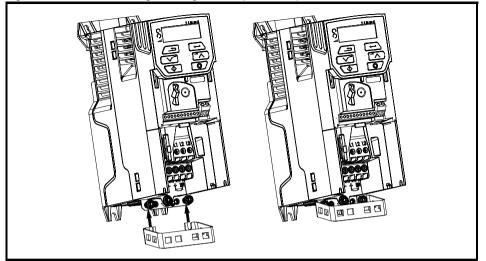
Loosen the ground connection screws and slide the grounding bracket in the direction shown. Once in place, the ground connection screws should be tightened with a maximum torque of 1.5 N m (1.1 lb ft).
