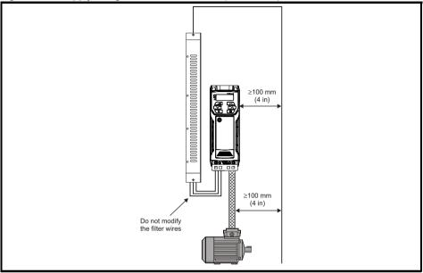
Figure 4-20 Sensitive signal circuit clearance
