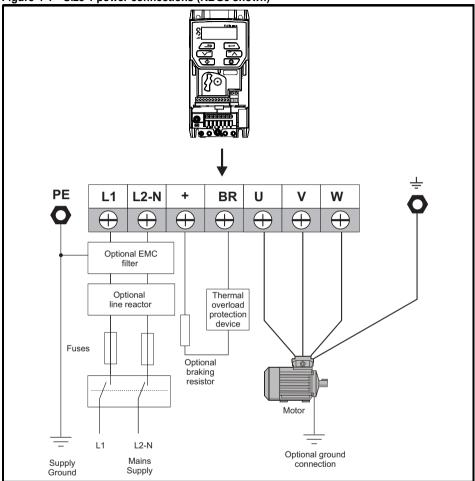
See Figure 4-5 Size 1 to 4 ground connections (KBG3 size 2 shown) on page 42 for further information on ground connections.
