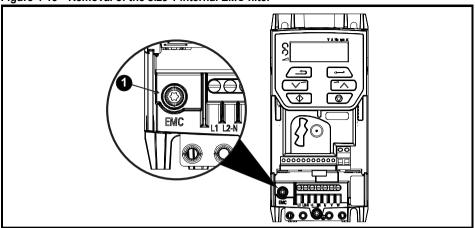
To electrically disconnect the internal EMC filter, remove the screw as shown above (1).
