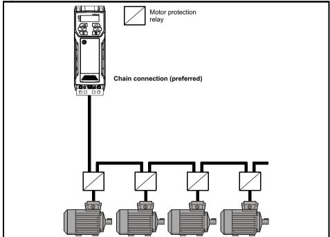
Figure 4-10 Alternative connection for multiple motors
