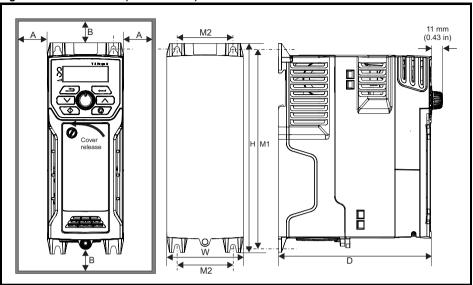
To remove the terminal cover, use a flat bladed screwdriver to rotate the terminal cover locating clip by approximately 30° in a counter clockwise direction, and then slide the cover down.
