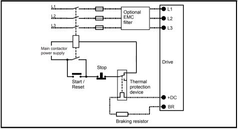
See Figure 4-1 on page 38 to Figure 4-4 on page 41 for the location of the +DC and braking resistor connections.
