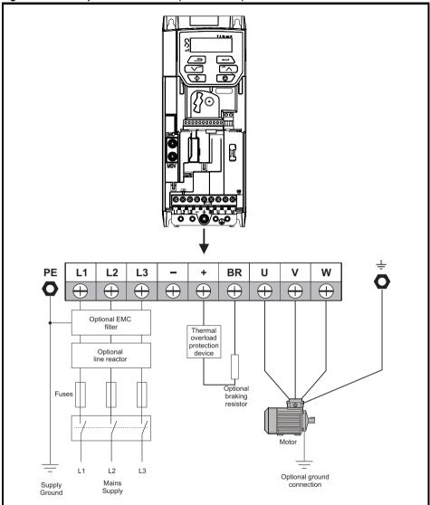
See Figure 4-5 Size 1 to 4 ground connections (KBG3 size 2 shown) on page 42 for further information on ground connections.
