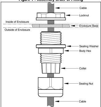
Figure 2 - Installed Fitting
