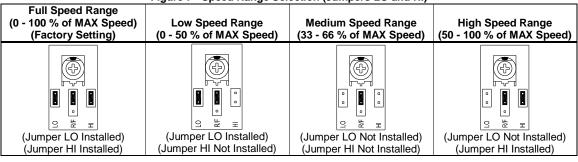
4.4 The speed for each preset can be fine tuned using the adjustable trimpots. All trimpots have been factory set for 50% speed. See Figure 8. (Note: The maximum speed is based on the MAX Trimpot setting.)
