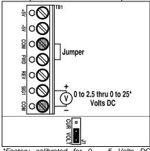
\*Factory calibrated for 0 – 5 Volts DC signal input.
