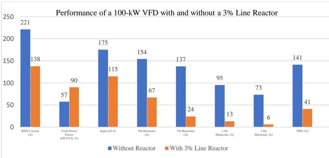
Figure 3. Performance of a 100-kW VFD without and with a 3% Reactor
