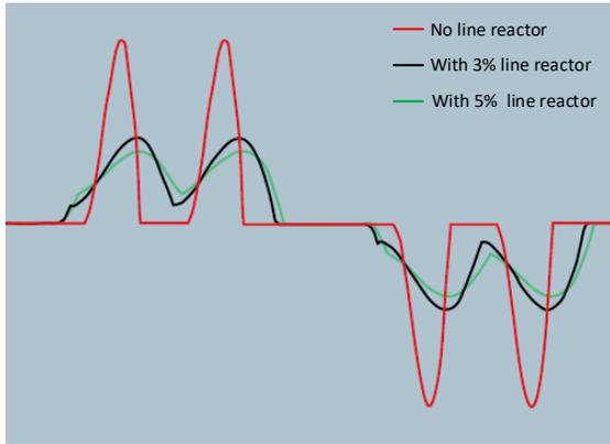
Figure 2. Line Current with and without Line Reactor
