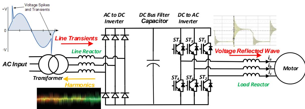
Figure 1: VFD and Motor System with Line and Load Reactors
