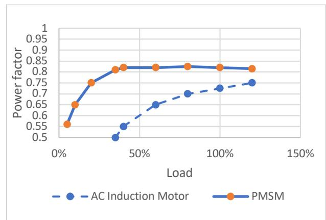
Figure 2: Typical AC Induction vs PMSM Power Factor
