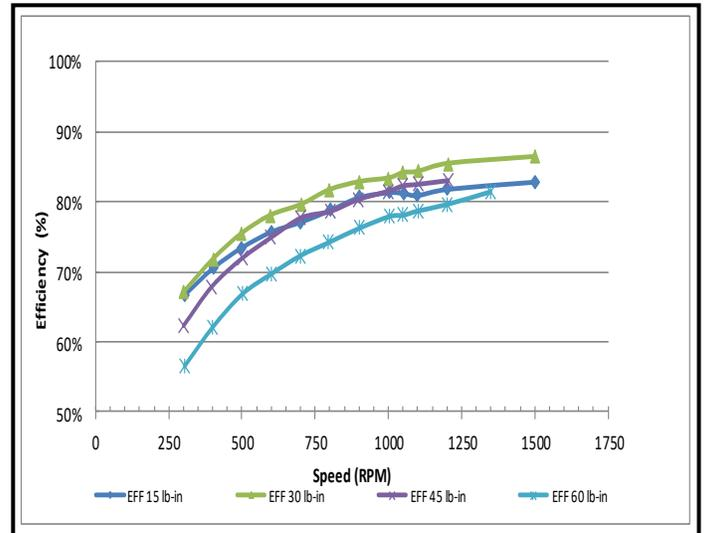
Figure 3: KBVF System Efficiency with a US Motors 1 HP PMSM
