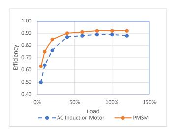
Figure 1:Typical AC Induction Motor vs PMSM Efficiency
