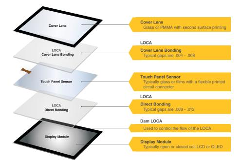
Liquid optically clear adhesive (LOCA) is a liquid-based bonding technology used in touch panels and display devices to bind the cover lens, plastic, or other optical materials to the main sensor unit or to each other.
