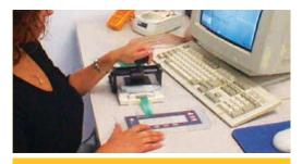
Figure 1: Recommended test setup.S witch tester measures: circuit continuity, closed-circuit resistance, LED polarity and function
