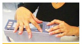
Figure 6a: NEVER burnish key or components during laminating assembly to well-mount.
