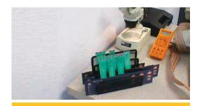
Figure 11: Detail view: showing membrane switches stacked vertically for testing prior to assembly. Never place objects on switches in unsupported manner.
