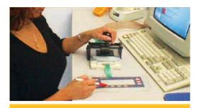
Figure 4b: NEVER actuate keys with any hard object.
