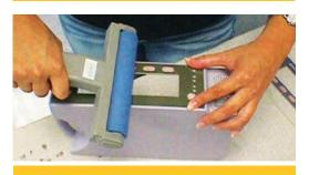
Figure 9: Using template, laminate membrane switch with smooth even pressure of hand-roller (typ. 40-45 Durometer, shore A)
