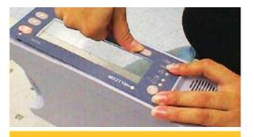
Figure 6b: NEVER burnish switch during assembly; it can inadvertently damage dome legs and/or SMT LEDs conductionads.
