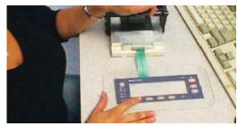
Figure 2a: Parts are tested prior to assembly. Note tactile membrane switch is laying flat in proper test fixture.
