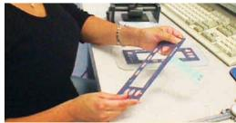
Figure 3a: NEVER actuate keys in unsupported position. Tactile membrane switches should ALWAYS be tested in flat (and supported for component clearance) position.
