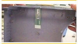
Figure 8: Detail side view: showing 0.040"polycarbonate template matching curve of well-mount in plastic casing.
