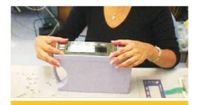
Figure 7d: Position template over partially laminated switch (ie., initial PSA tack, not completely laminated)
