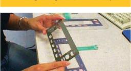
Figure 7b: Align template over membrane switch for proper orientation.
