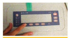
Figure 2b: Detail view: tactile membrane switch is laying flat in proper test fixture during test key actuation.
