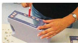
Figure 10: Even after assembled, NEVER actuate keys with hard object. Only actuate keys with human finger-tip.
