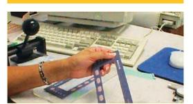
Figure 3b: NEVER actuate keys in unsupported position.
