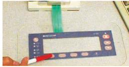
Figure 4a: NEVER actuate keys with any hard object (pen, sylus, etc.)Membraneswitch keys are designed b be actuated withhuman finger tip.
