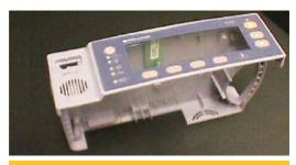
Figure 12: Finished part laminated to typical customer casing. Membrane switches may ONLY be laminated to substrate ONE time. VIS can not warranty parts that have been removed and/or repositioned for final assembly.
