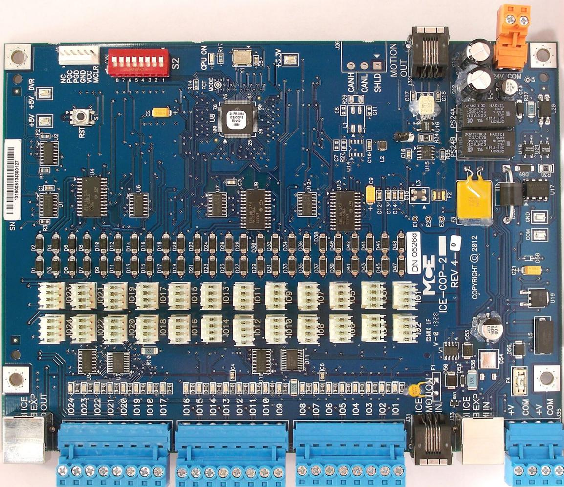
**MC-CPI-2 Car Panel Interface Board** Converts the Discrete closures from car panel buttons and switches to CAN data and passes it through the Landing System Interface board (MC-LSI) to the car controller or dispatcher.
