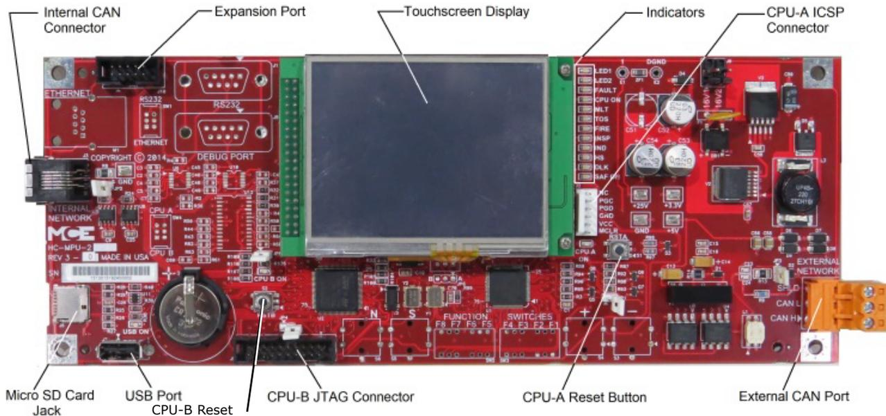
Figure 5.1 shows the indicators, push buttons and terminals on the main processor unit.
