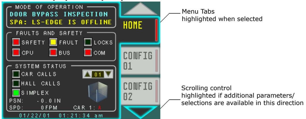
On the Home display screen, **tabs** to the right of the window show what additional adjustment, control, and diagnostic screens are available. Up and Down arrows scroll through the tabs. To access a screen, simply touch the associated tab.
