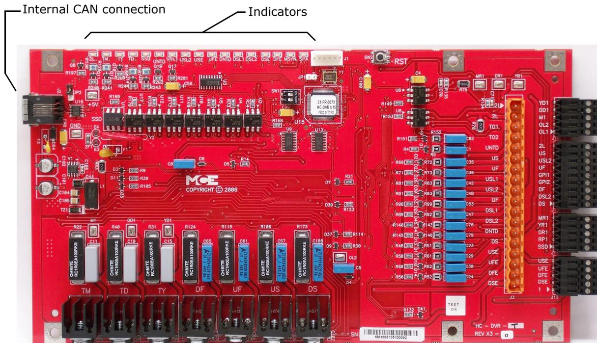
Starter, valve and hoistway limit connections
