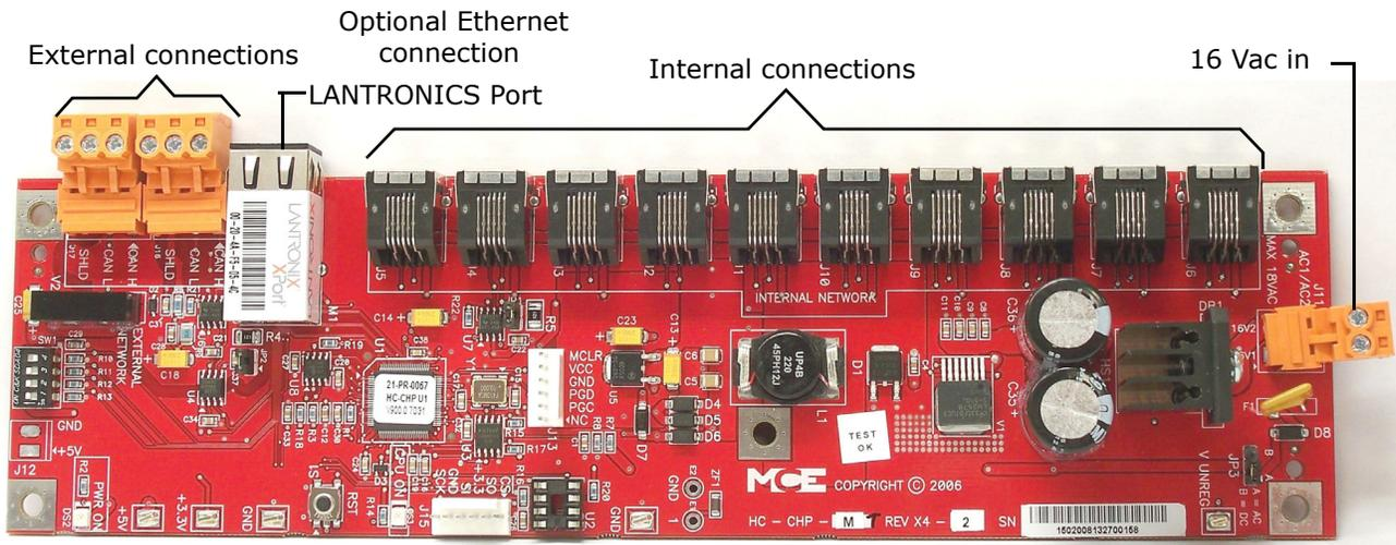
**HC-MPU-2-TS Main Processor Unit** Performs control data processing. The HC-MPU-2-TS is responsible for car operation, car communication, programming and diagnostics, redundancy monitoring, system software validation and duplexing. For more information see [“HC-MPU-2-TS Main Processor Board”](#) on page 6-15.
