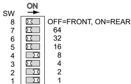
When setting addresses, use the values silk screened on the circuit board, not those shown on the DIP switch.
