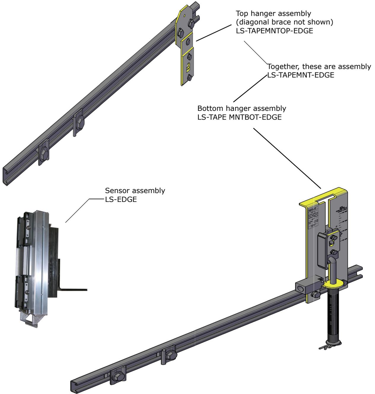
Steel tape, magnets & connecting cables not shown
