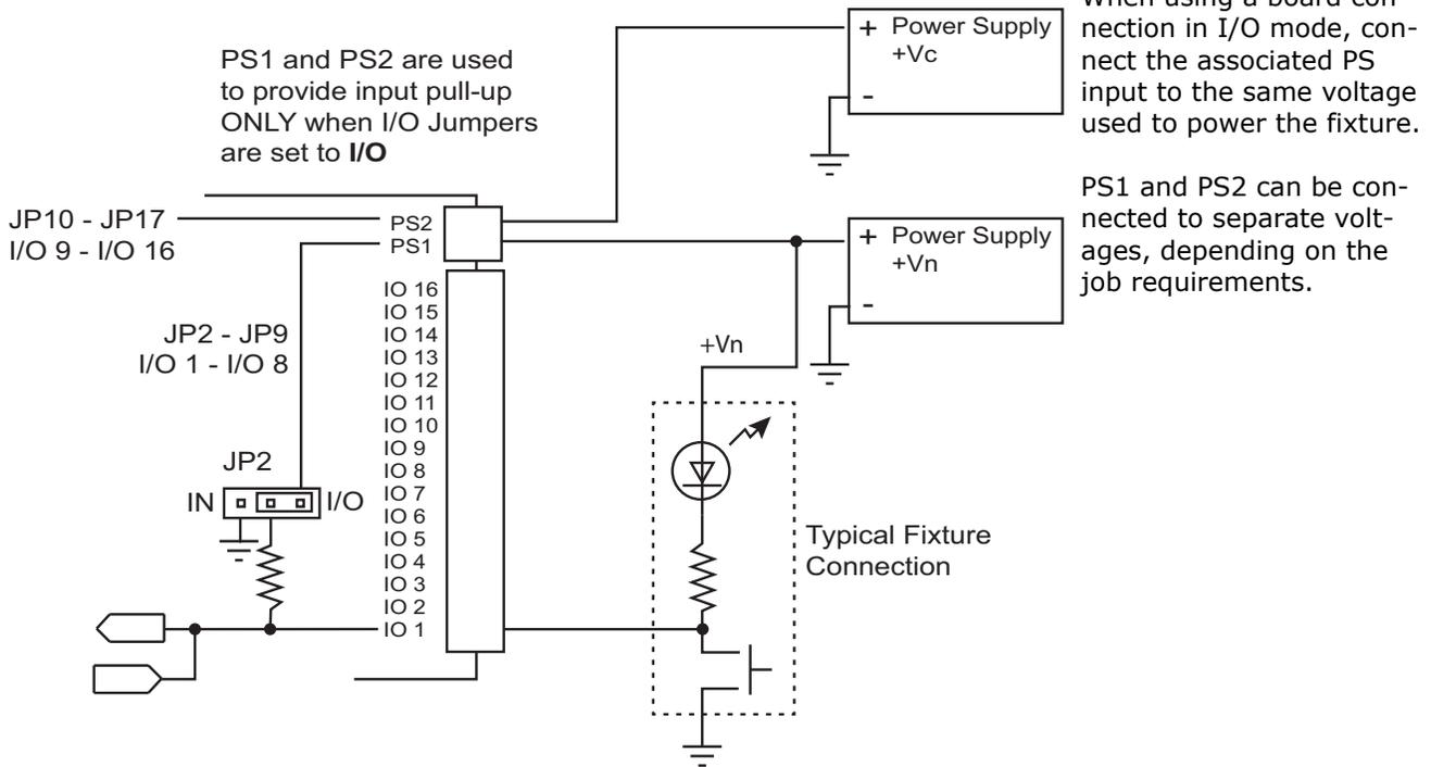
Figure 6.8 Typical Input or Output Connection (Board ID 32 to 36)
