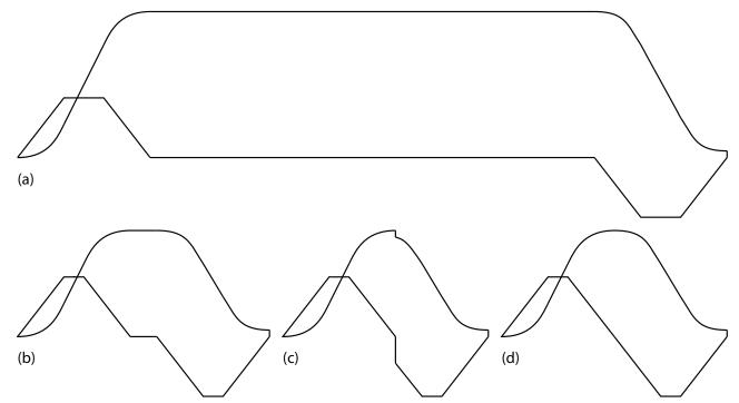
Velocity and Acceleration: (a) profile at contract speed; (b) insufficient lag compensation with profile at less than contract speed; (c) excessive lag compensation with profile at less than contract speed; (d) optimum lag compensation with profile at less than contract speed.
