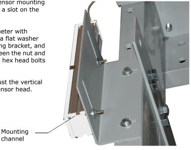
Alternatively, you can use 8 x 32 channel nuts and screws or 1/4" square head bolts and nuts. However, if you are inserting the screws toward the body of the sensor, you must be very careful that you position spacers to prevent the screw from damaging the sensor.
