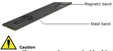
The arrows on the magnetic side of the tape must point in the up direction and face the car.
