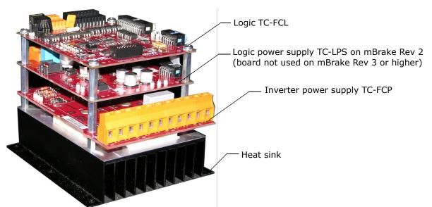
Figure 5.19 TC-FCL Board - Configuration
