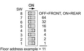
When setting addresses, use the values silkscreened on the circuit board, not those shown on the DIP switch.
