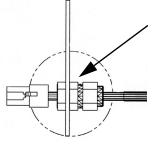
The NEMA 4X / 12 version provides strain relief and sealed entry using a gasketed cover and special hardware as shown.
