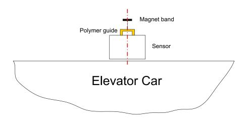
2. Remove the front polymer guide from the sensor by flexing it slightly out at the center and pulling it from the retaining clips at each end. Leave the sheet-plastic membrane in position on the sensor.
