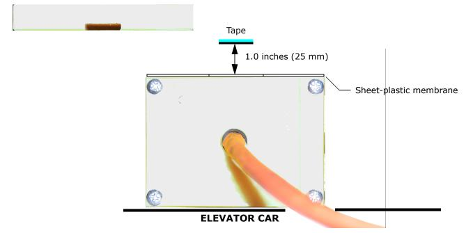
4. Re-attach the polymer guide with the tape resting in the guide slot.
