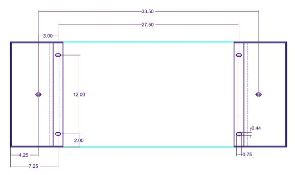
Dimensions for attaching base feet of Standard NEMA 1 enclosure (16" deep x 42" wide)
