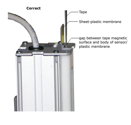
With the sensor guide re-installed, the tape should arc gently away from the car at the top and bottom, forcing the steel side of the tape firmly against the polymer guide.
