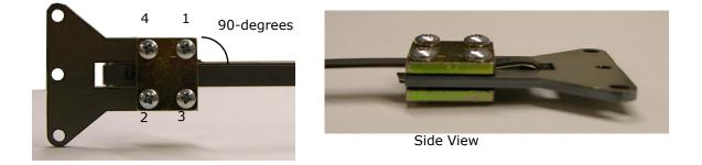
3. In the same 1, 2, 3, 4 order, make several passes, tightening each screw just a little each time. Finally, torque each screw to 14 in-lb. or 224 in-oz. (depending on the units on your torque driver).
