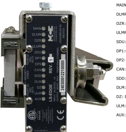
MAIN: Sensor processor A active. DLMR: Down Level Marker (Rear). DZR: Door Zone (Rear). ULMR: Up Level Marker (Rear). SDU: Slow Down Up. DP1:Quadrature pulse. DP2: Quadrature pulse. CAN: CAN communication activity. SDD: Down Slow Down. DLM: Down Level Marker (Front). DZ: Door Zone (Front). ULM: Up Level Marker (Front).
