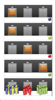
**Destination based dispatching** results in a low mix of destinations per car, requiring fewer stops and less time.
