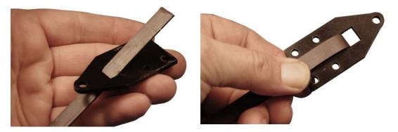
3. Place the tapped clamping piece on the back, and the through-hole piece on the top of the end piece. Hold with one hand, insert, and gently tighten one of the securing screws.
