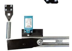
3. The assemblies to which the tape attaches, both top and bottom, allow fine alignment adjustment without having to work with the heavy, rail clamp hardware. After adjustment, torque the 3/8 bolts/nuts to 10 ft lbs.
