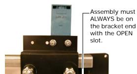
7. Move the switch to the outer mounting position. The switch must be properly aligned and the mounting screws torqued to 15 to 17 in-lbs.
