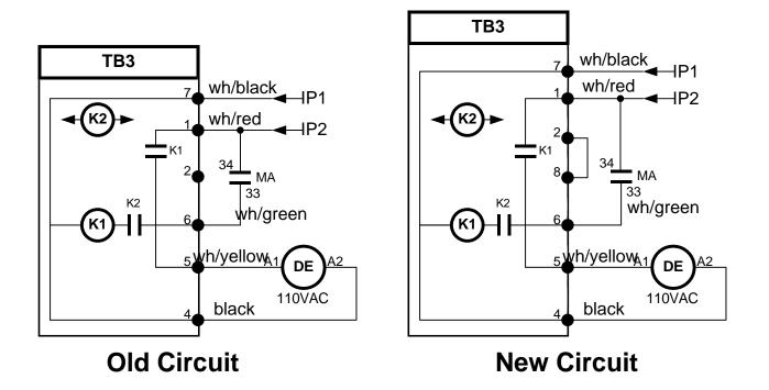
After installing the jumper on TB3-2 to TB3-8, refer to the "Relays Section" of the prints. Locate the "Drive Fault" contact on this page.
