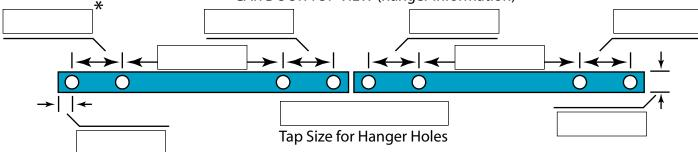
\* Standard center to center dimension for MCE door hangers is 4 1/8". An adapter is used to accommodate other center to center dimensions. If adapters are used, the door track must be raised 1/2" to compensate.
