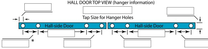
\* Standard center to center dimension for MCE door hangers is 4 1/8". An adapter is used to accommodate other center to center dimensions. If adapters are used, the door track must be raised 1/2" to compensate.
