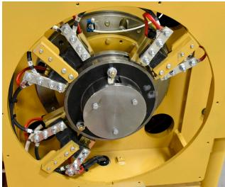
Figure 1-2 Rotor Assembly
