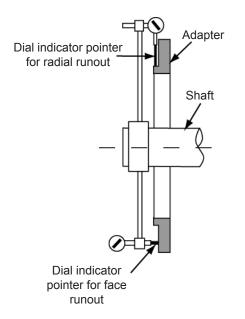
Figure 2-3: Generator adapter check
