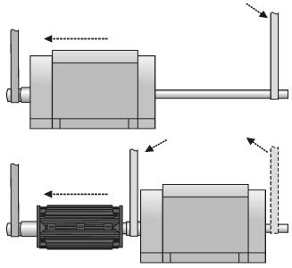
Figure 5-7:Rotor Removal
