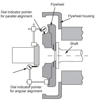
Figure 2-4: Alignment check
