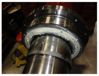
Figure 5-6: Bearing Installed on Shaft
