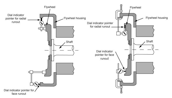
Figure 2-1: Flywheel housing check
