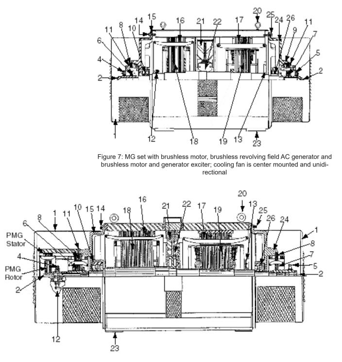
Figure 8: MG set with brushless motor, brushless revolving field AC generator and dual brushless motor and generator exciter, and permanent magnet generator (PMG)
