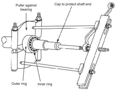
Figure 6: Removing the bearing
