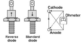
Figure 2: Testing rotating rectifiers with an ohmmeter
