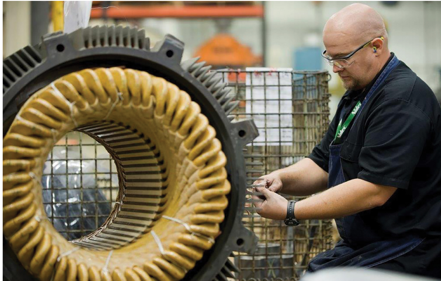
Employee wiring stator in Mena, AR plant.
