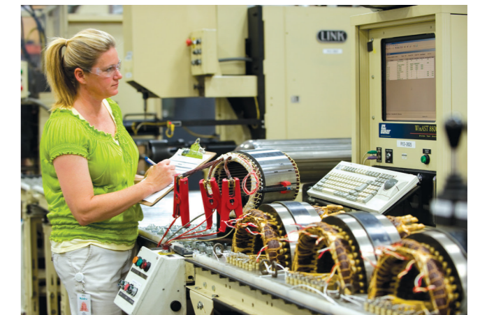
Employee inspecting stators in Mena, AR plant.
