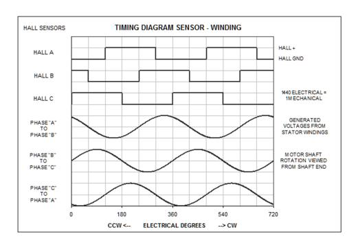
In order to properly commutate the Merkle-Korff 2.25" BLDC motor, the following table is provided to indicate the required motor phase state for a given hall-effect state.
