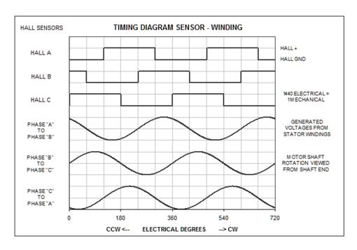
In order to properly commutate the Merkle-Korff 2.25" BLDC motor, the following table is provided to indicate the required motor phase state for a given hall-effect state.
